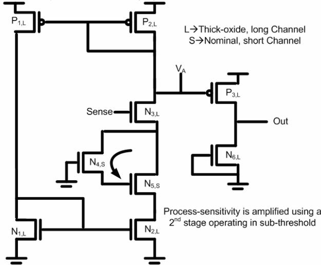
Fig 2: Process-Variation Sensor for NMOS devices
