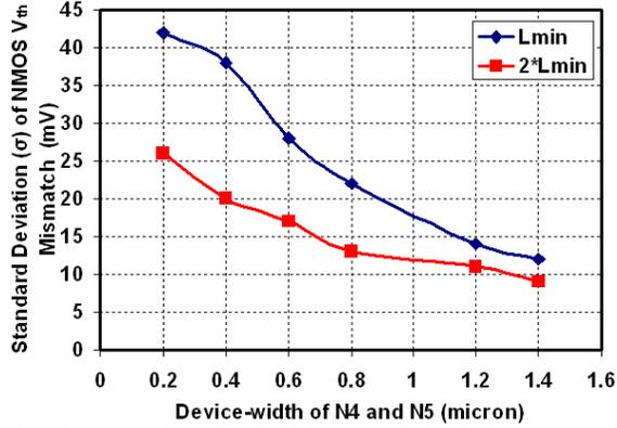
Fig 10: Impact of device-width on standard deviation of  $V_{th}$  mis-match
