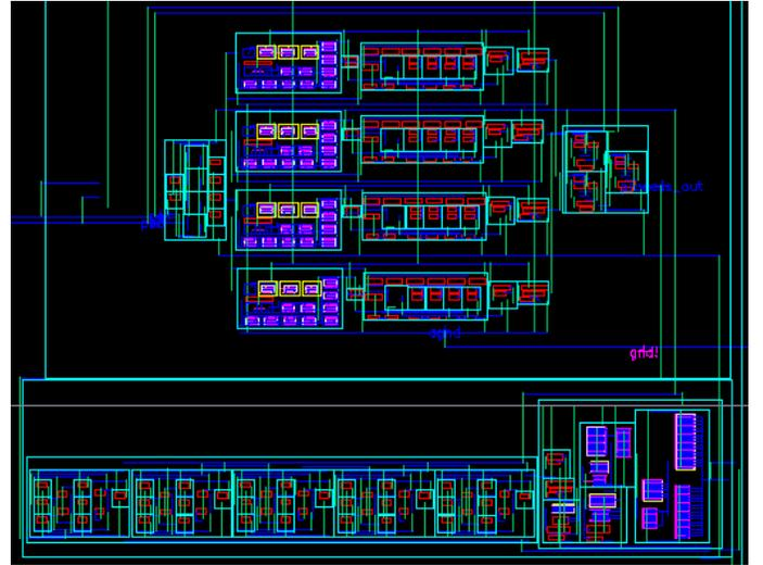
Fig 12: Layout of test-setup for process-sensors. Layers M1, M2 and M3 used for metallization. Sensors and digitization blocks are at the top while the frequency-divider and buffer-horn are at the bottom
