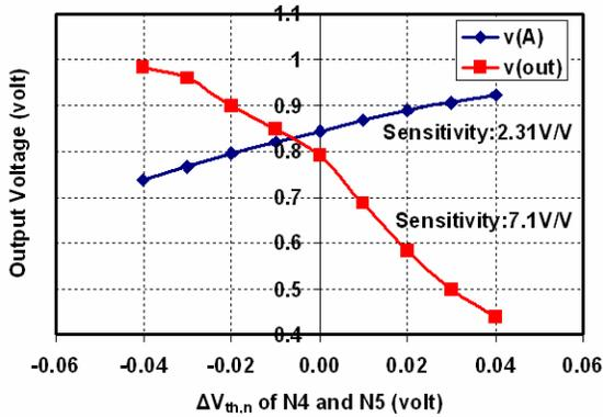
Fig 3: Sensitivity of NMOS process-variation sensor
