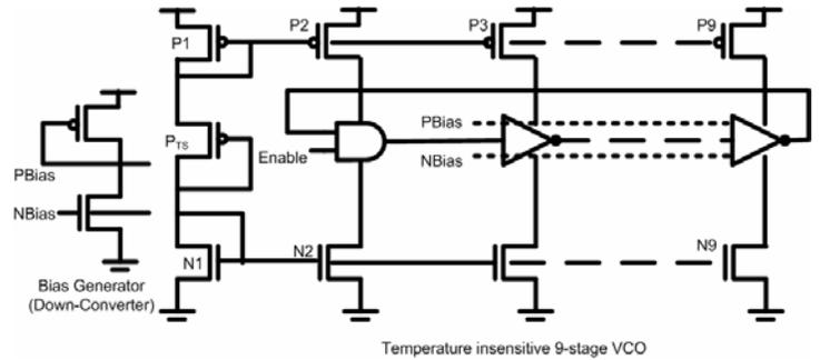
Fig 4: Digitization using temperature-insensitive current-starved 9-stage VCO (V<sub>OUT</sub>=NBIAS)
