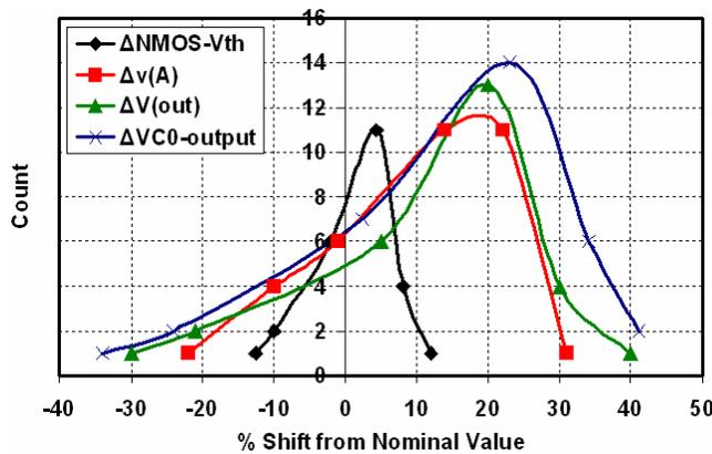
Fig 7: Histogram of % shift from nominal value of nodes at various stages of NMOS  $V_{th}$  sensing
