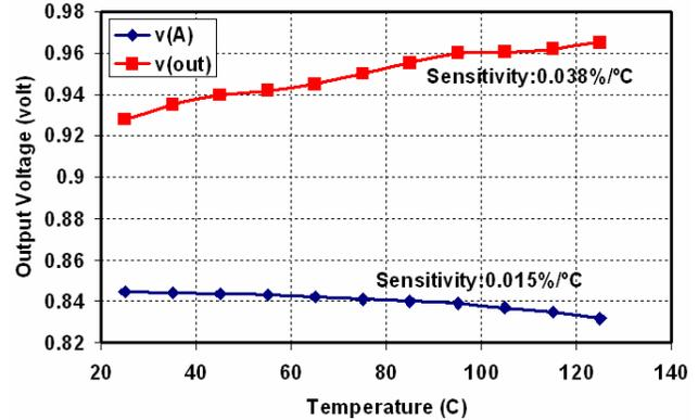
Fig 8: Process-sensor response to temperature variations
