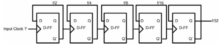
Fig 5: Divide-By-32 Ripple Divider
