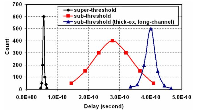
Fig 1: Delay distribution of a 15-stage ring-oscillator for different operating modes and device-types
