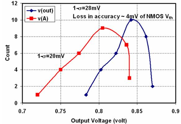
Fig 9: Histogram of sensor output in the presence of supply-noise
