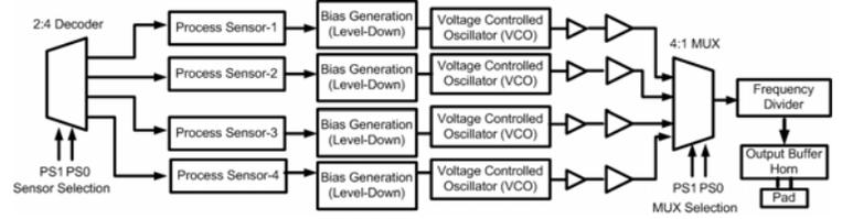
Fig 11: Test setup for proposed process-sensor using 45nm IBM-SOI toolkit provided by MOSIS
