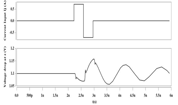
Figure 4: Voltage response at  $z$  from current load at  $j$
